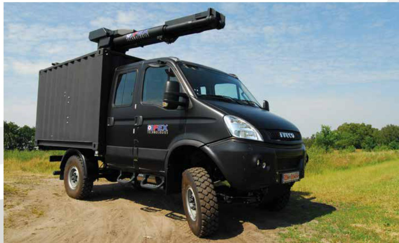
IFEX® firefighting system on IVECO cross-country vehicle
