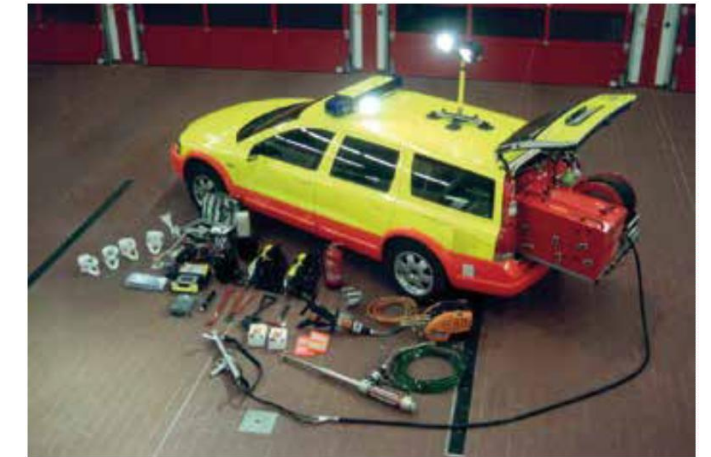
These vehicles equipped with the IFEX® firefighting system are used by the Hamburg fire brigade in the Elbe tunnel.
