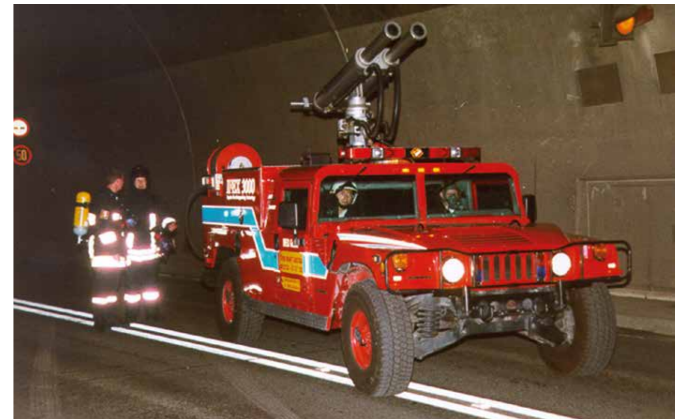
Hummer as an emergency vehicle for tunnel fires (2x12 litres Dual-Intruder)
