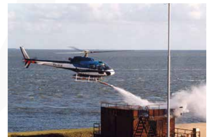
IFEX® Helicopter in the firefighting application (2x18 litres Dual-Intruder)
