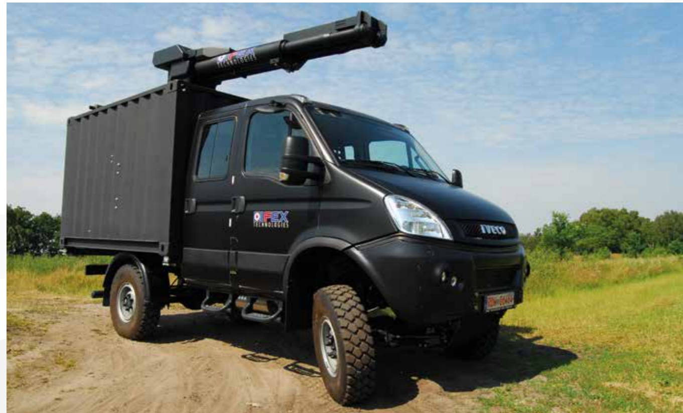
IFEX®-firefighting system on IVECO cross-country vehicle
